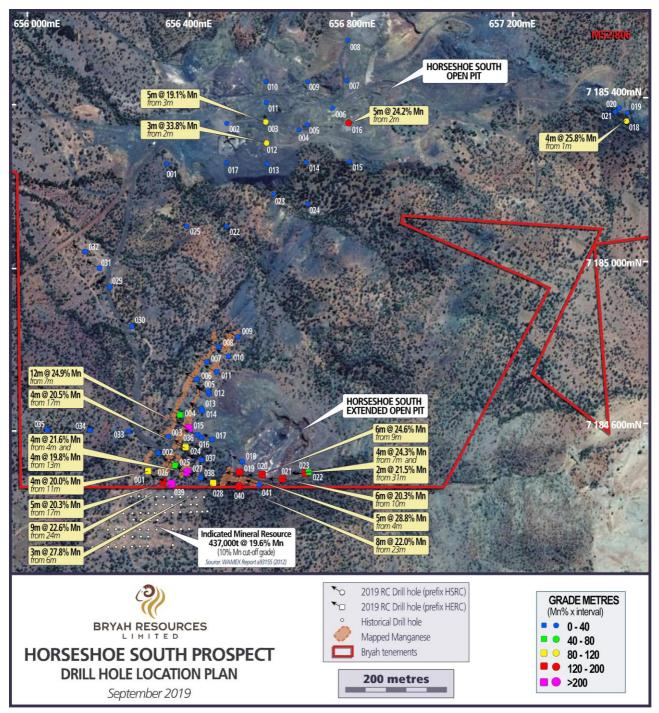
Figure 4 - - Drill hole Location Plan - Horseshoe South
