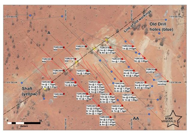
Figure 1: Drill collars and traces with significant intercepts
