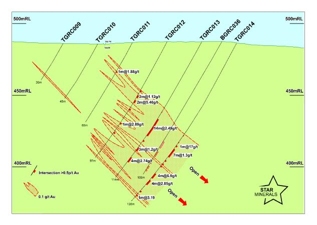
Figure 2: Cross section TGRC009 to TGRC014 with significant intercepts within 0.1g/t mineralised envelope
