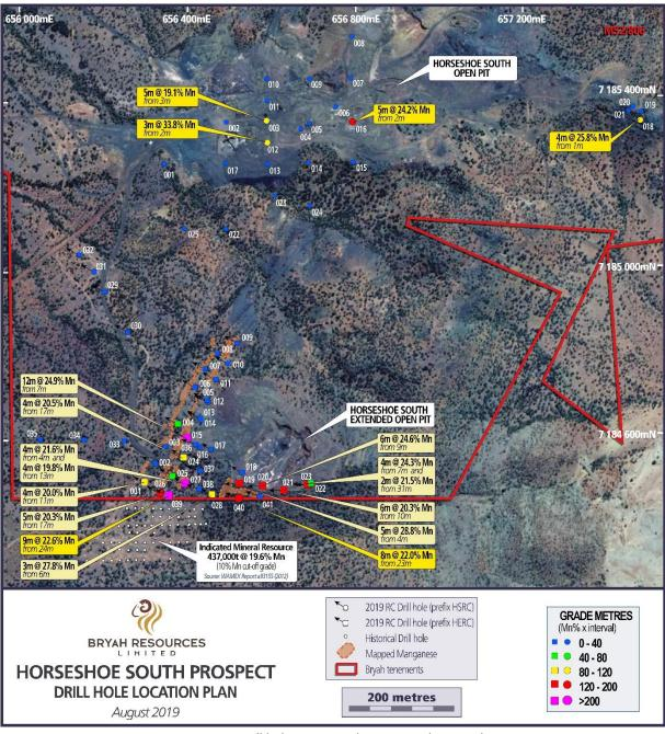
Figure 1 – Drill hole Location Plan – Horseshoe South.
