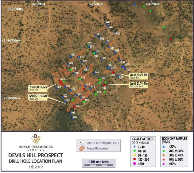
Figure 6 – Drill hole Location Plan – Devils Hill.
