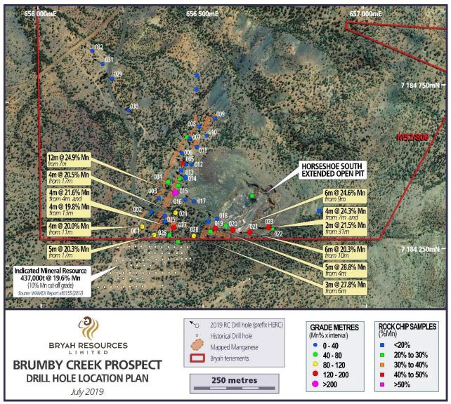
Figure 5 – Drill hole Location Plan – Horseshoe South.
