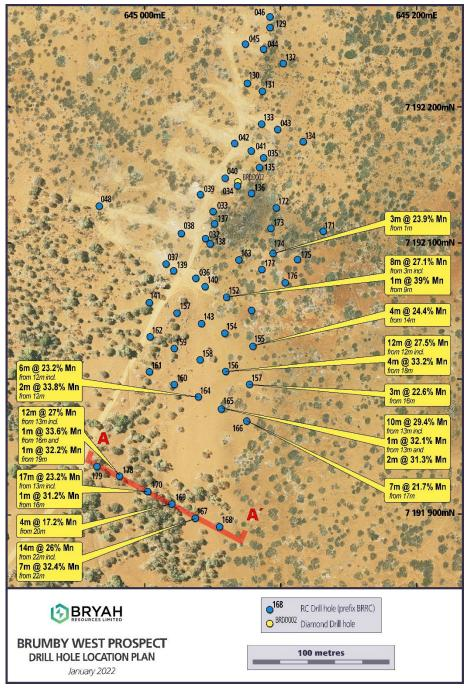
Figure 5 6 Collar Plan of Drilling at Brumby West with location of Drill Section
