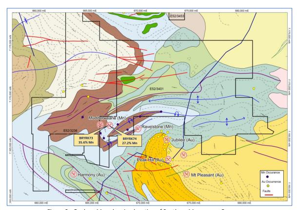
Figure 3 - Geology Map showing location of Southern Manganese Occurrences including Mudderwearie Manganese Mine (refer to legend in Fig 1).
