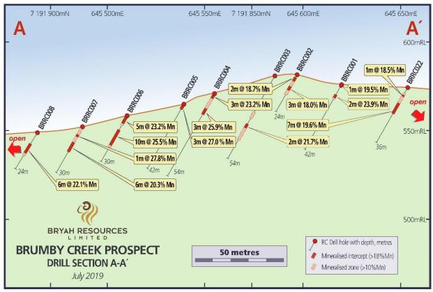
Figure 3 – Drill hole Section AA' – Brumby Creek.
