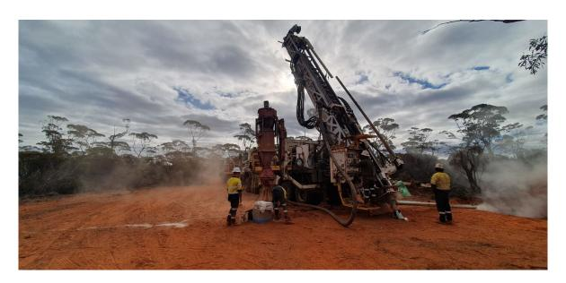
Figure 1 RC drill rig on the first drill hole at Pegasus
