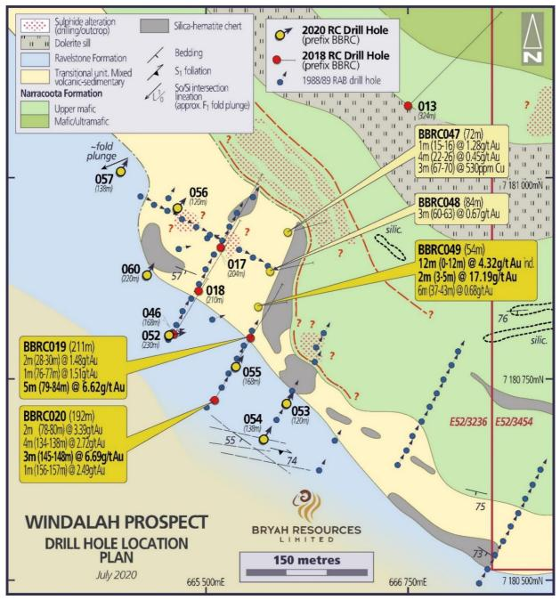
*Figure 2 - Windalah Prospect - Drill Hole Location Plan over interpreted bedrock geology.*
