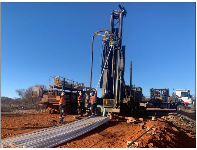
Figure 6 - Drill rig crew commence casing BBRC050 with 50mm PVC pipe
