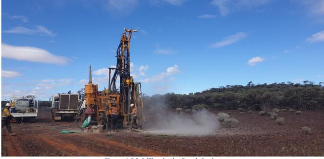
Figure 1 RC drilling in the Bryah Basin
