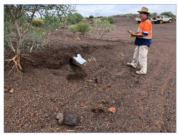
Plate 7 - Rohan Williams sampling remnant manganese stockpiles at East Mudderwearie Mine This sample recorded an assay of 16.3% Mn.
