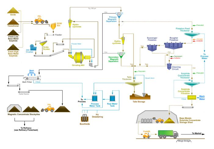
Figure 15 Concentrator Flowsheet Schematic
