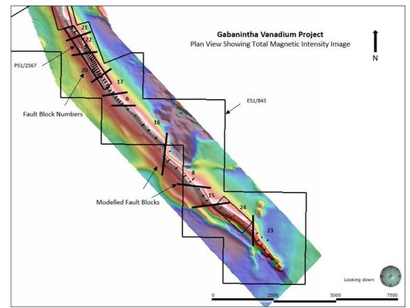
Figure 7 Plan View showing Fault Block Locations at Gabanintha
