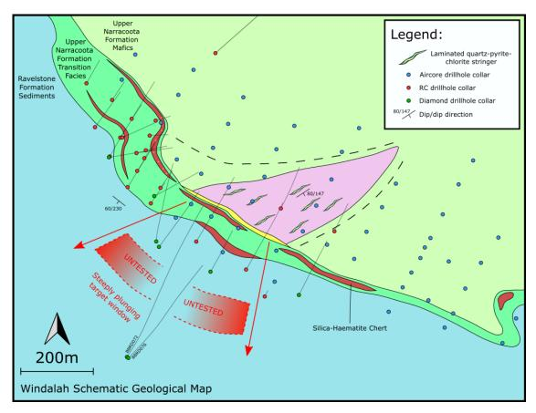
Figure 8: Schematic geological map of the Windalah prospect showing the plunging target zone and BBRD072 and BBRD076.
