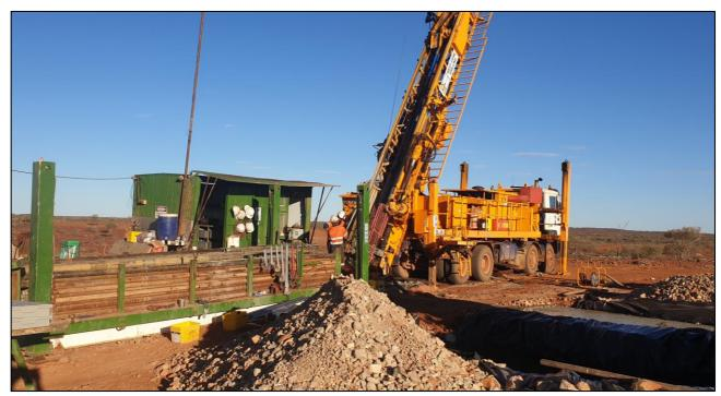
Plate 1 – Diamond Drill Rig on site at Tumblegum South
