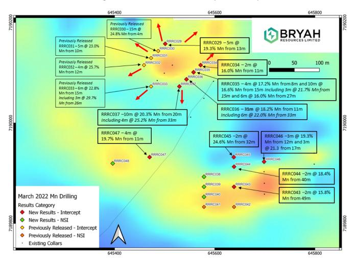
Figure 4 Redrum Results on 2021 GAIP survey chargeability heat map
