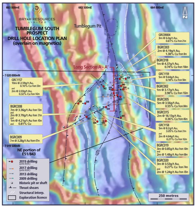
Figure 2 – Drill Hole Location Plan
