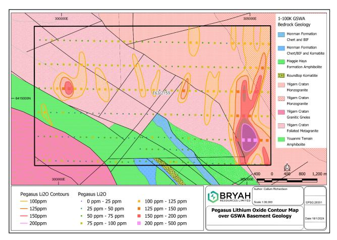
Figure 1 - Pegasus soil sampling anomaly map with Li₂O contours shown over GSWA 1:100,000 Interpreted Basement Geology Map.
