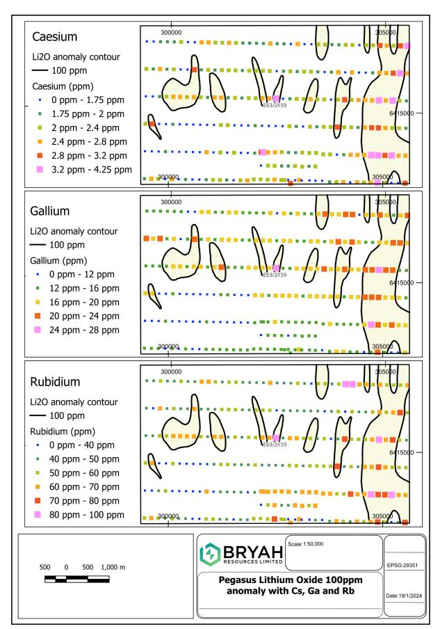
Figure 2 – Caesium, Gallium and Rubidium soil geochemistry maps with Li<sub>2</sub>O +100ppm anomaly shown
