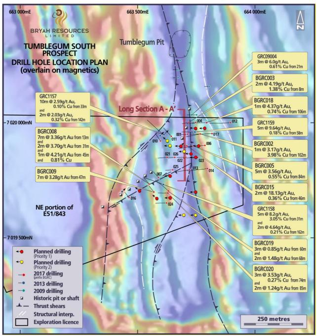
Figure 2 – Drill Hole Location Plan
