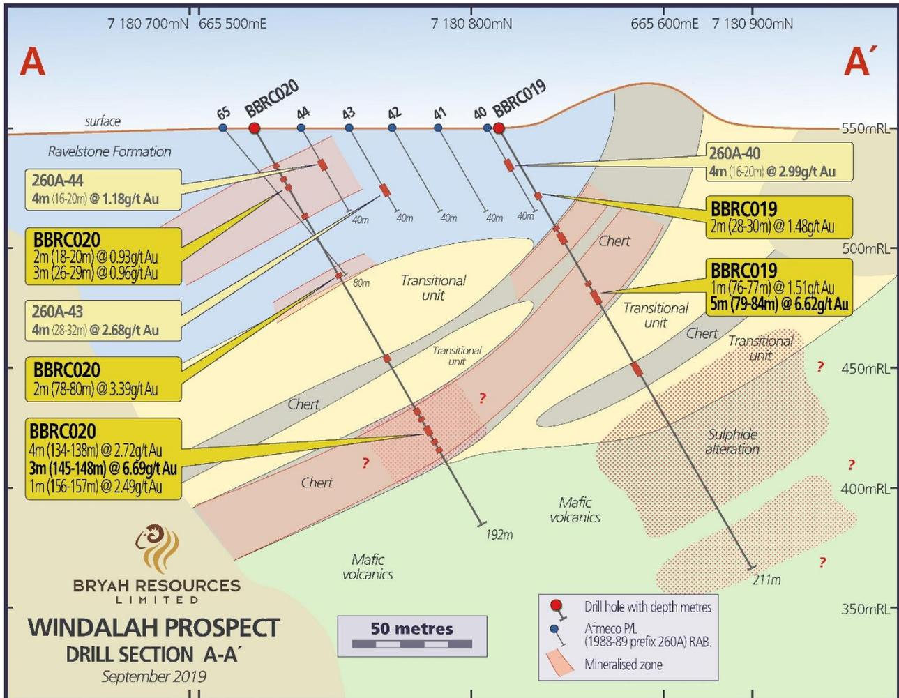
Figure 4 – Drill Section A-A'
