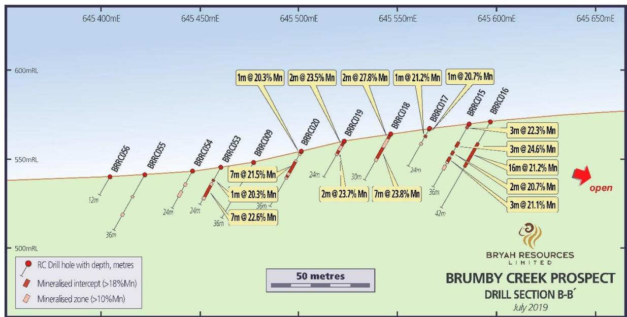
*Figure 8 - Drill hole Section BB' – Brumby Creek.*
