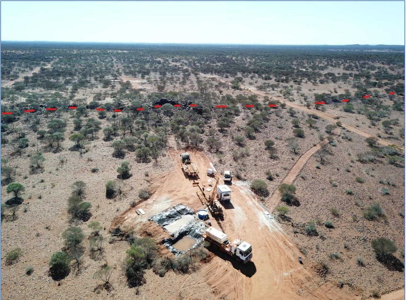
*Plate 1 – Diamond drill rig set up on RC pre-collar hole BBRC064. Red dashed line marks outcropping chert contact, which separates the overlying Ravelstone Formation sediments (in foreground) from the underlying volcanic Narracoota Formation (in background).*
