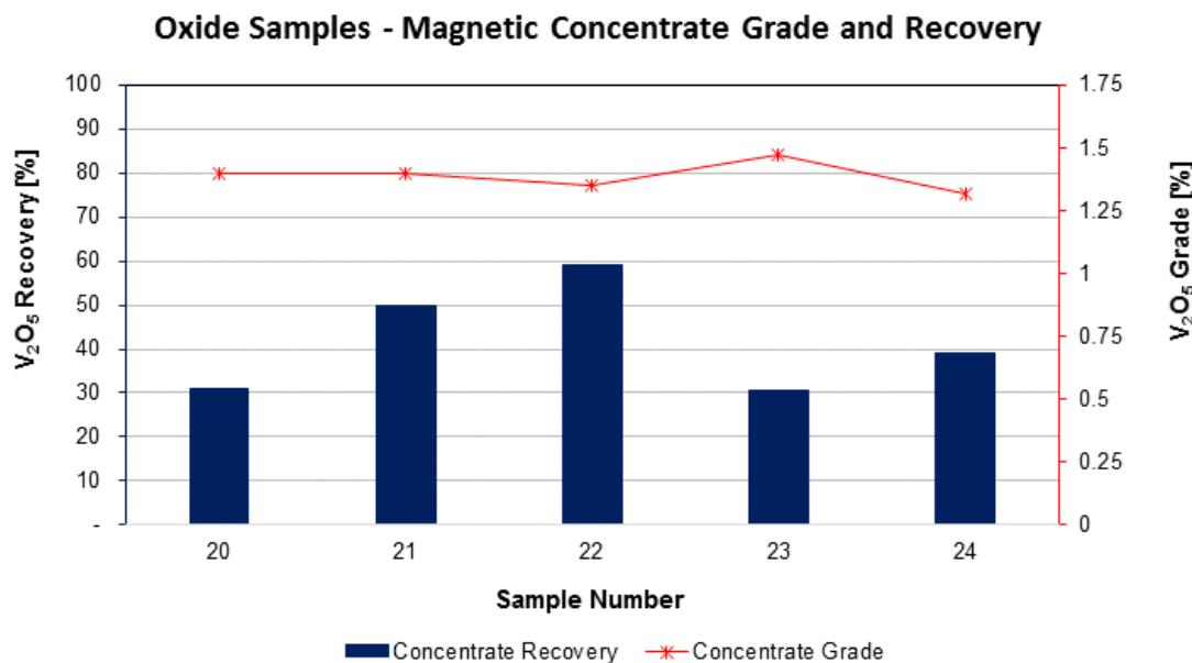
Figure 7 V<sub>2</sub>O<sub>5</sub> recovery and concentrate grade for magnetic separation tests on oxide high grade metallurgical samples
