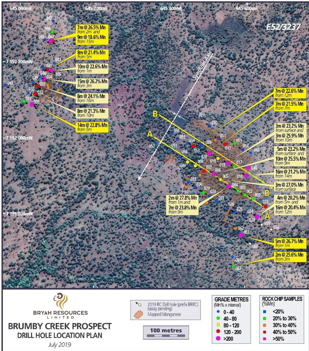
Figure 2 – Drill hole Location Plan – Brumby Creek.
