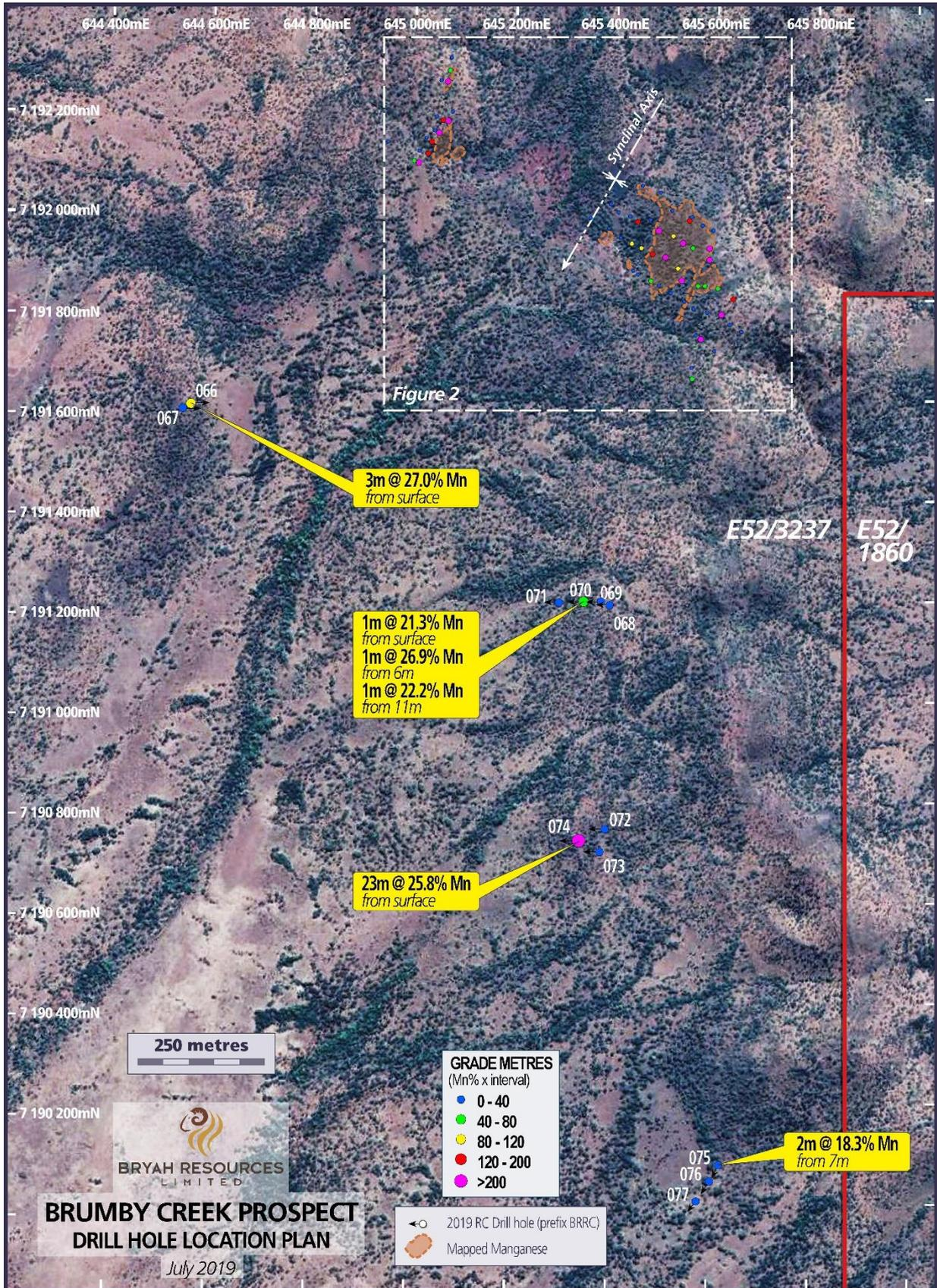
Figure 3 - Drill hole Location Plan – Brumby Creek.
