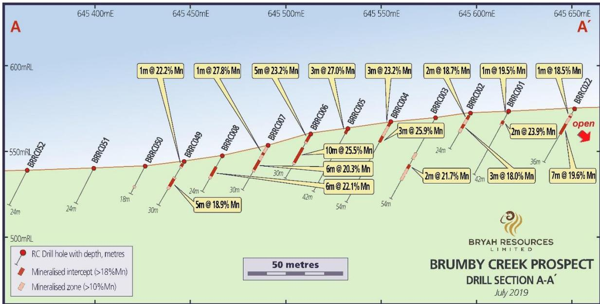
Figure 4 – Drill hole Section AA' – Brumby Creek.
