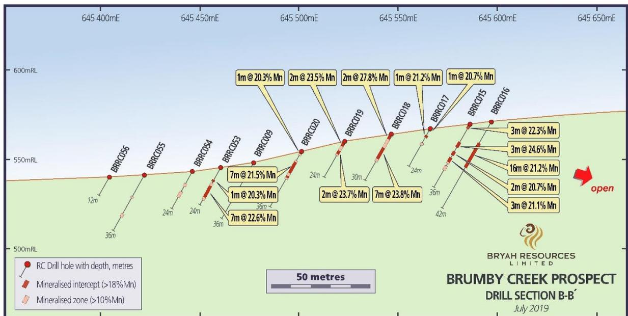
Figure 5 - Drill hole Section BB' – Brumby Creek.
