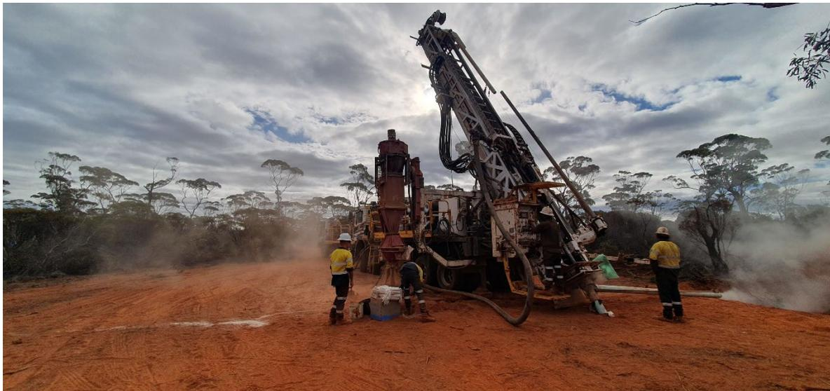
Figure 1 RC drill rig on the first drill hole at Pegasus
