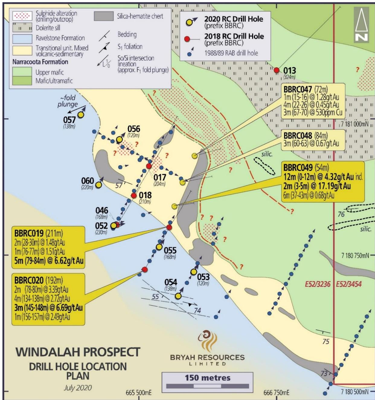
Figure 2 - Winalah Prospect - Drill Hole Location Plan over interpreted bedrock geology.
