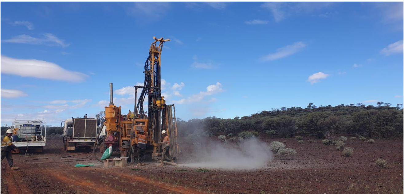
**Figure 1 RC drilling in the Bryah Basin**
