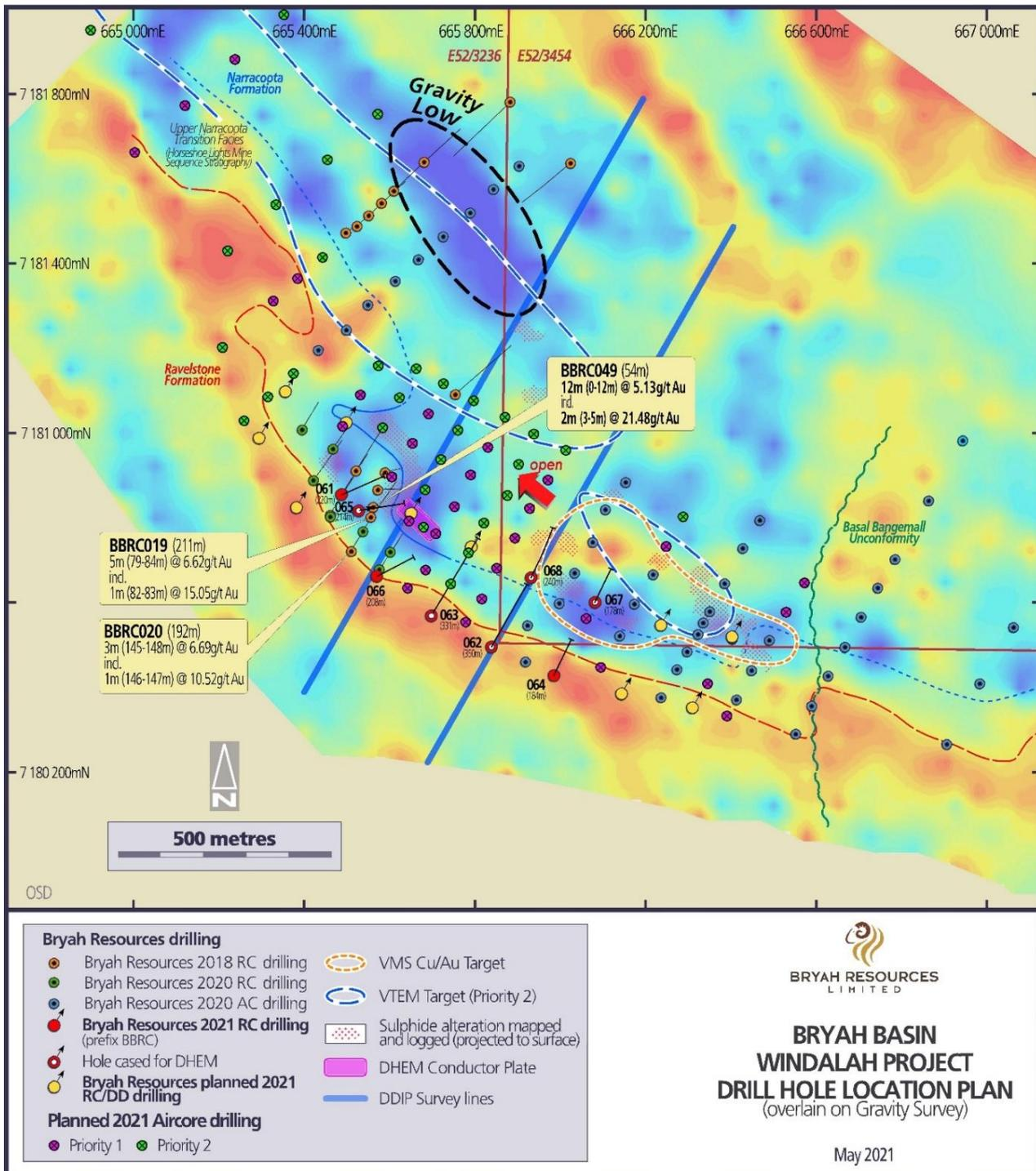
Figure 2 – Windalah Prospect Drill Hole Location Plan
