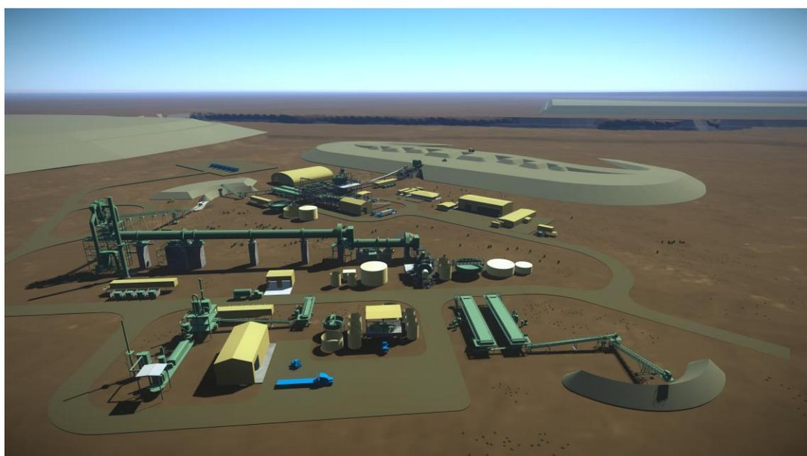
**Figure 3 Plant Layout (Aerial view looking east. Processing plant in the foreground, IWL to the left (north). The ROM blending stockpiles are visible behind the plant and the Gabanintha open cut (3.2 km long) is in the background. A second waste dump is located east of the pit.**
