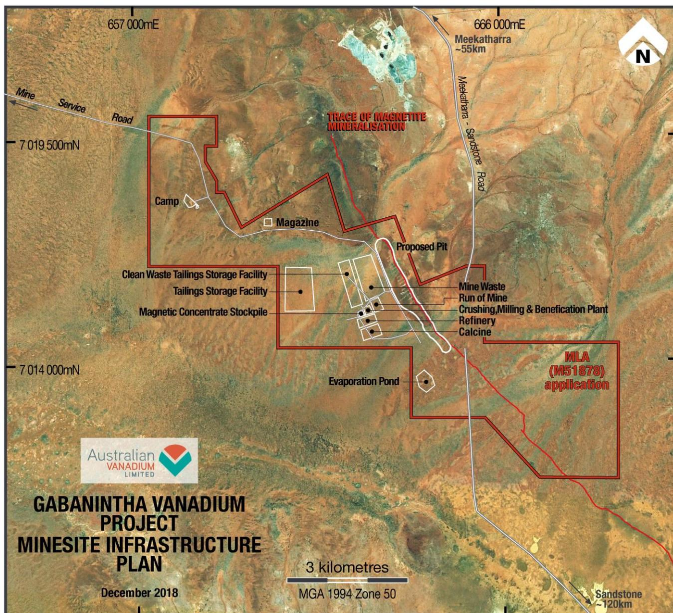
**Figure 17 Infrastructure Location Diagram (Initial Proposed) Gabanintha Project**
