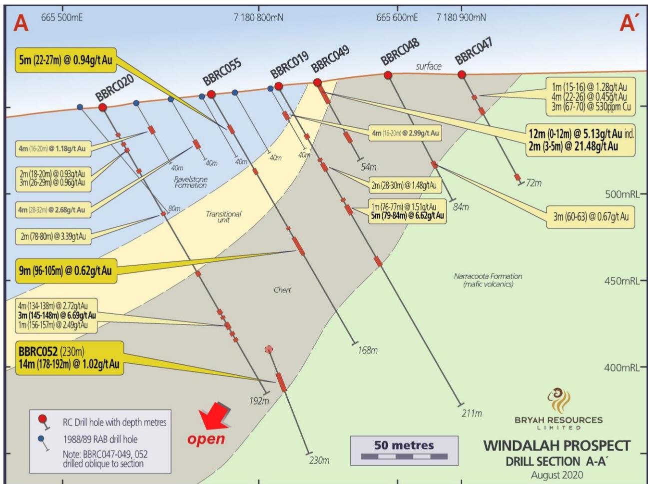
Figure 3 - Windalah Prospect Drill Section A-A'
