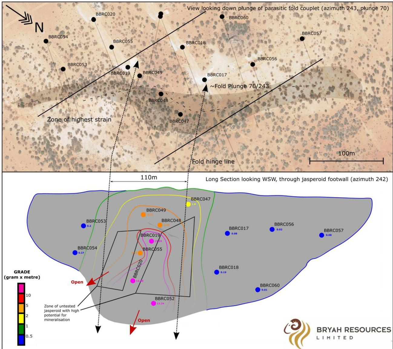
Figure 4 – Schematic Long Section looking WSW
