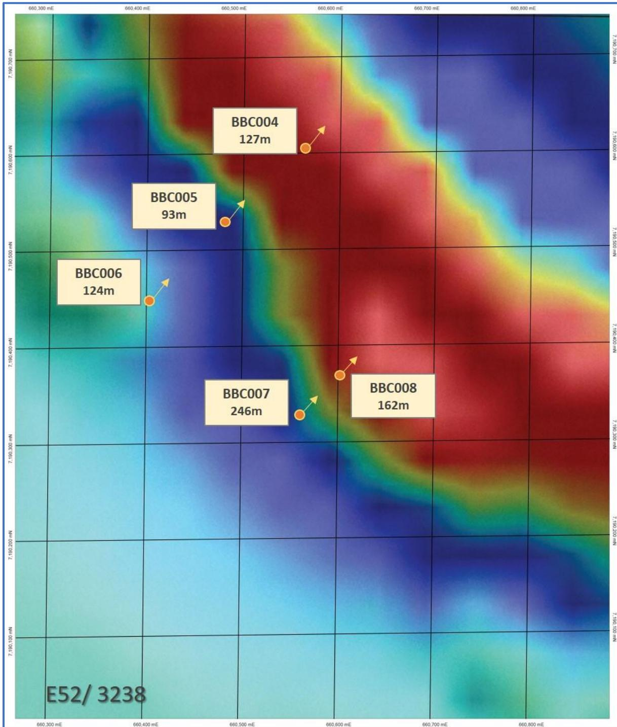
Figure 2 – Jupiter Prospect Drill hole location plan overlain on VTEM image (Ch30 1vd NE sun)
