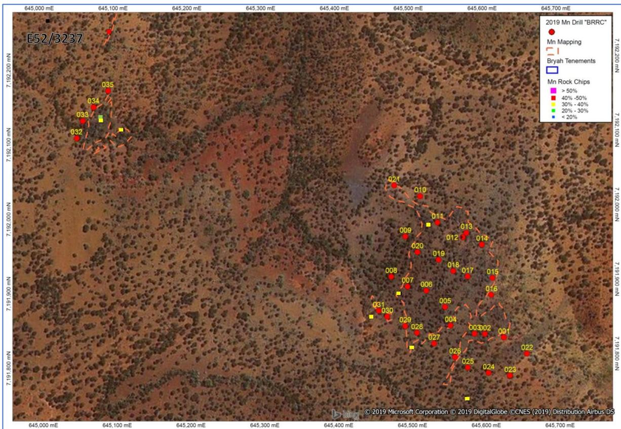
Figure 4 – Drill hole Location Plan – Brumby Creek.
