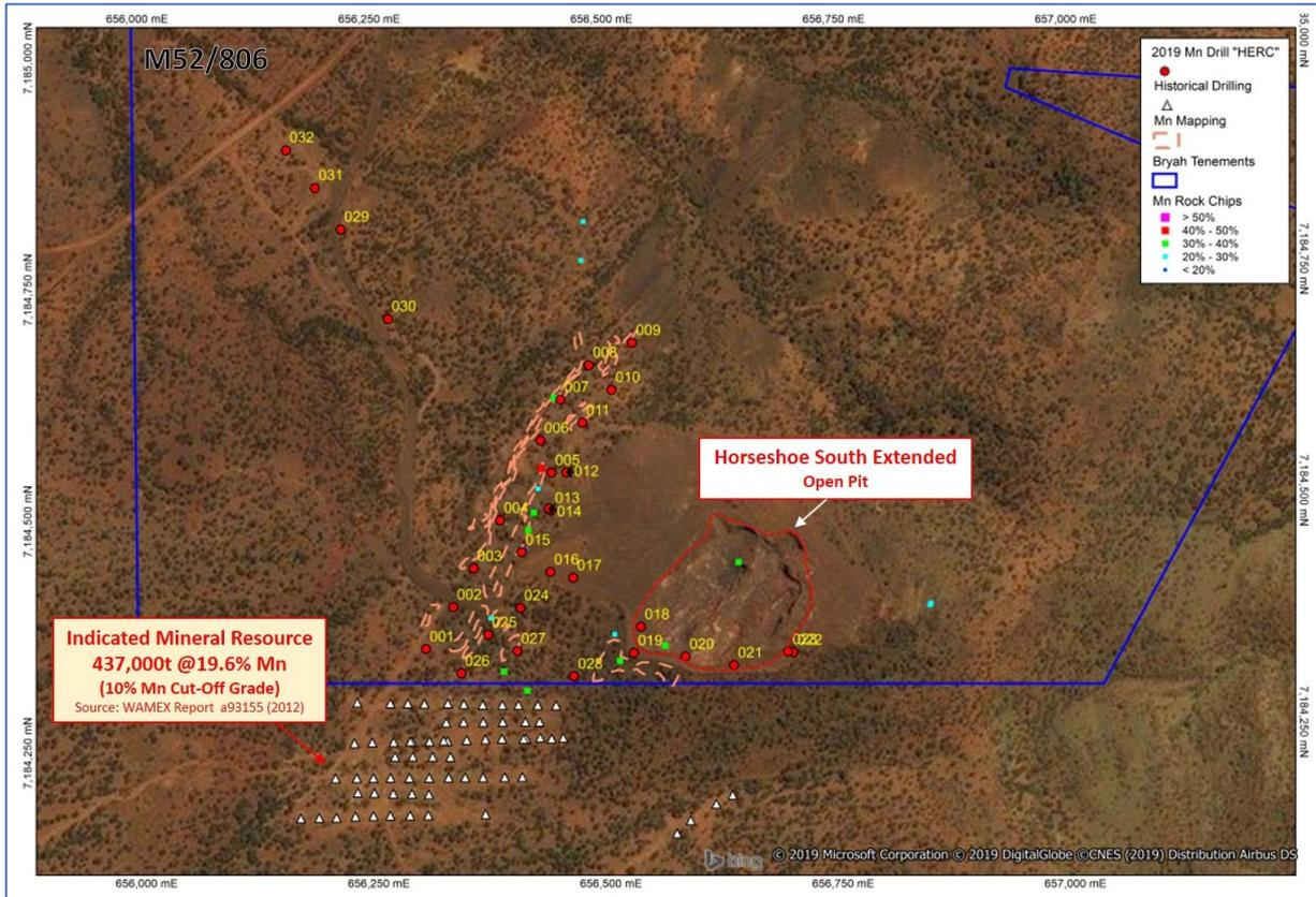
Figure 3 – Drill hole Location Plan - Horseshoe South.
