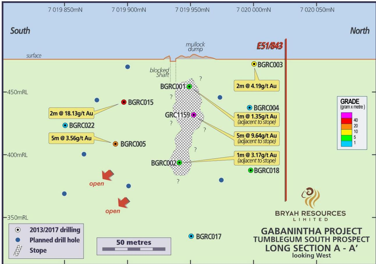
Figure 3 – Long Section A-A'
