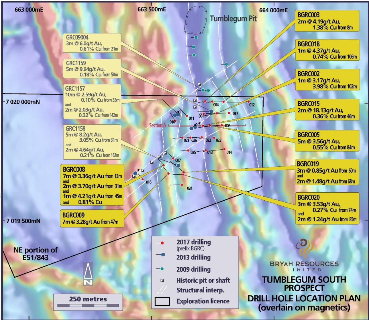
Figure 6 – Tumblegum South Drill Hole Location Plan
