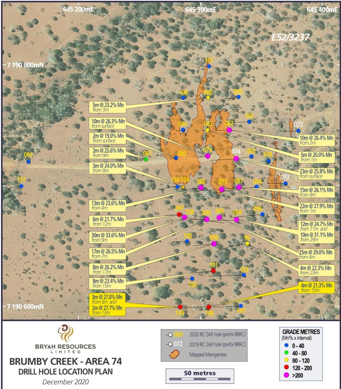
Figure 5 – Brumby Creek - Area 74 Drill Hole Location Plan
