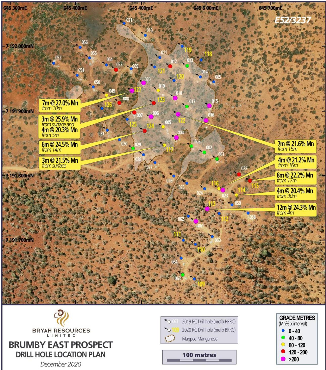
Figure 3 – Brumby East Prospect Drill Hole Location Plan
